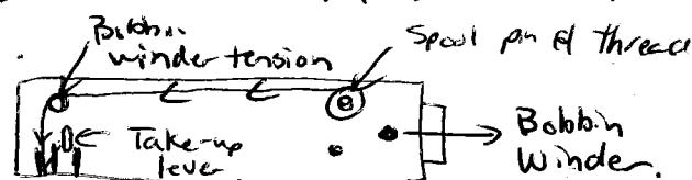
B 2) Floss into the bobbin winder tension, it is the silver bar across the width of the machine that has arrows coming out of it & an upside down "J". After that make sure to go into the thread guide (the hook on the top).
