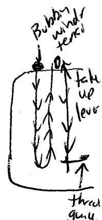
A&B 4) Go around the back of the take-up lever to put the thread into the "eye of the bunny".
